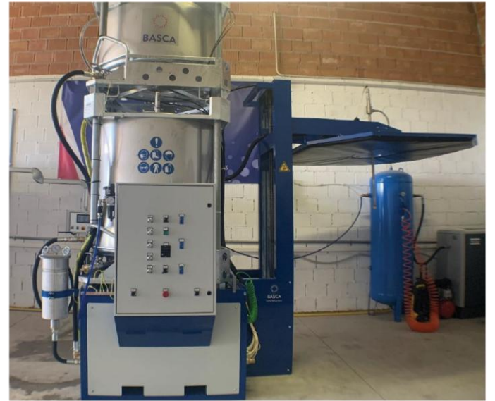
POT WASHING MACHINE FOR A 50% SLUDGE REDUCTION
