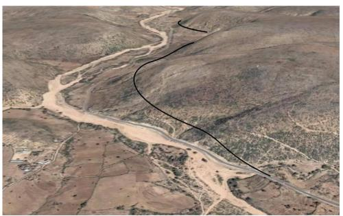
Figure 4-18 Alternative roadway alignment out of flood limits
