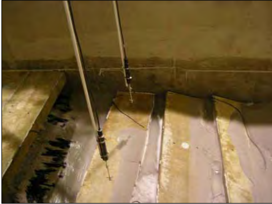
Figure 8.13. Laboratory tests of the weir-flow damage mechanism showing scour has continued to point of undermining failure of 3 sections (6 feet) of roadway surface. (USA/TAMU flume tests, June 2005).
