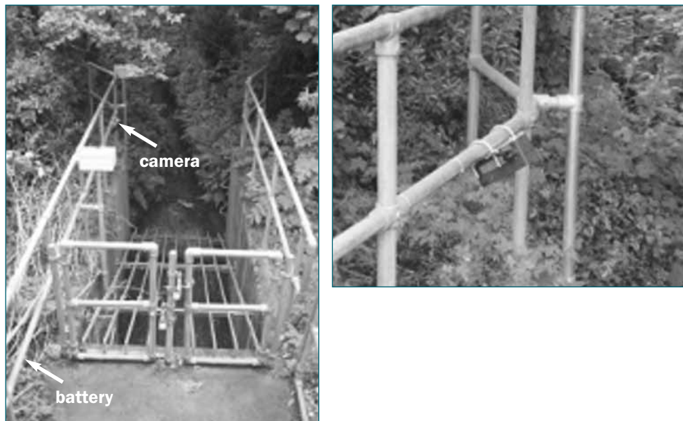
Figure A3.8 Camera sited on railing
