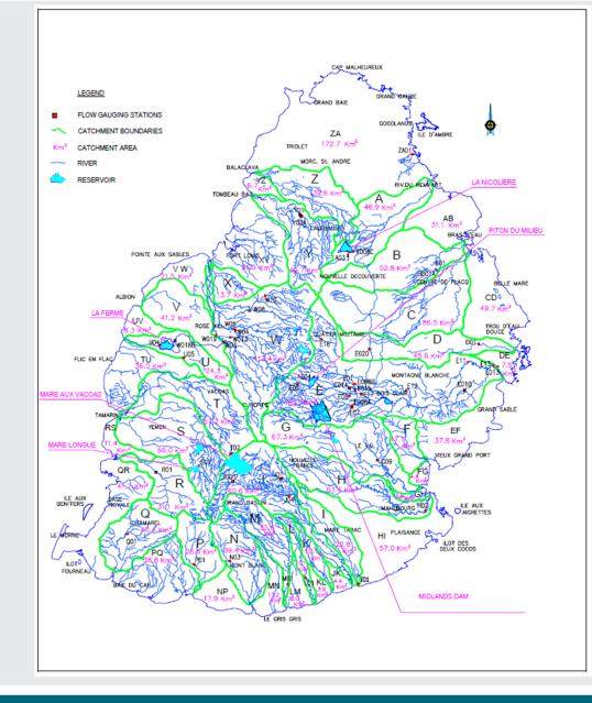
Rational method often used for smaller areas Q = 0.278 C.I.A Q ~ discharge m<sup>3</sup>/s C ~ Runoff coefficient I ~ Rainfall intensity mm/hr A ~ Area km<sup>2</sup>
