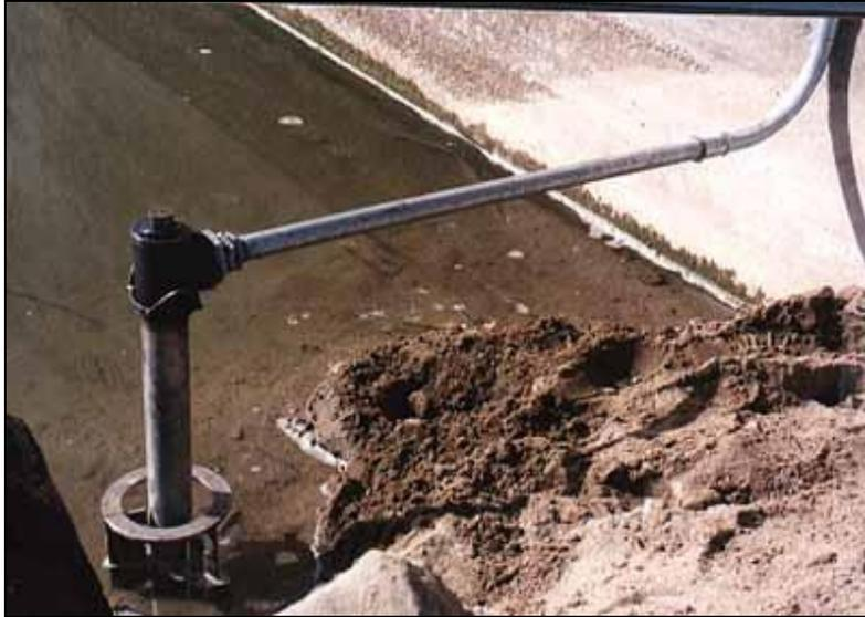
Figure 9.16. Detail of magnetic sliding collar on the streambed.
