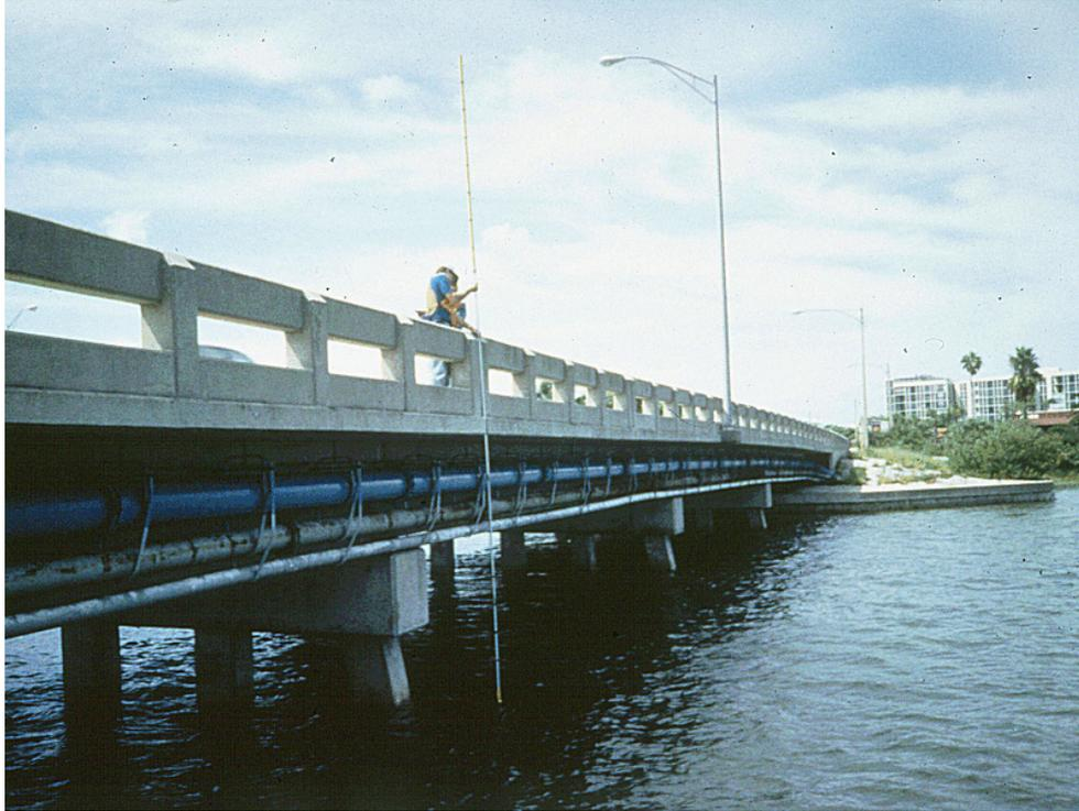
Figure 9.1 Sounding pole measurement.
