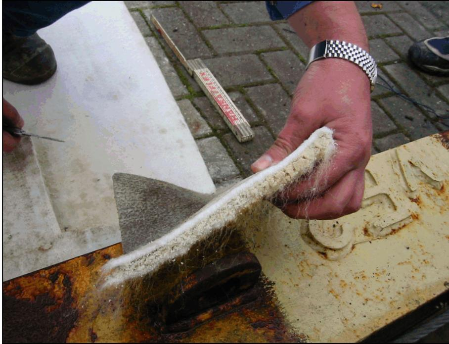
Figure 5.2. Close-up photo of SandMat™ geocomposite blanket.
