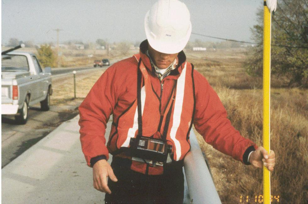
Figure 9.3. Portable sonar in use.
