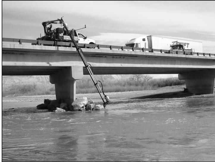
Figure 9.9. Sonar instrument deployed from articulated arm truck.
