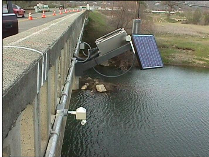
Figure 9.18. Tilt meter on California bridge.
