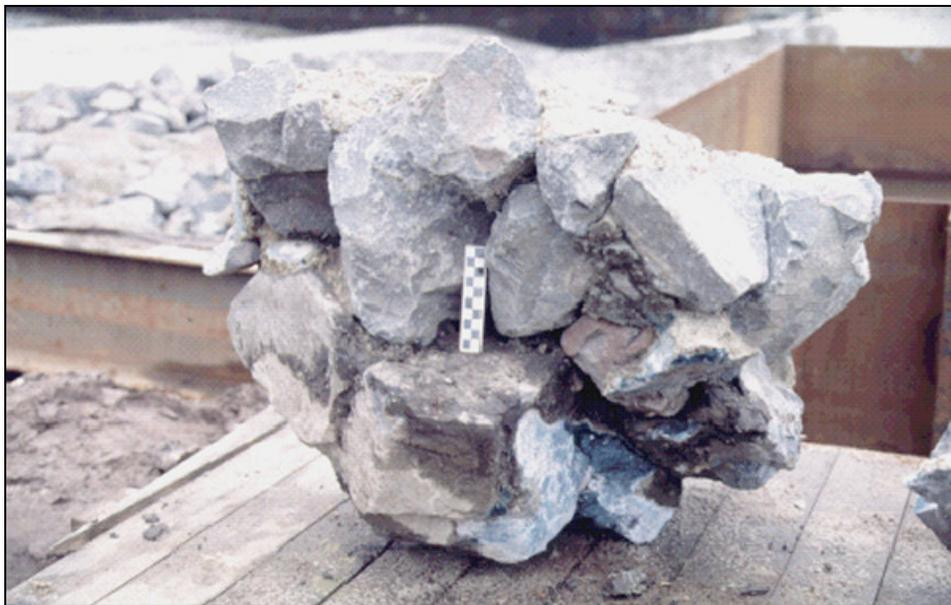
Figure 5.21. "Conglomerate" of partially grouted riprap, Federal Waterway Engineering and Research Institute, Karlsruhe, Germany (Heibaum 2000).
