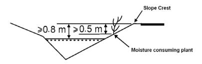
Fig. 4. Drainage class 1 (redrawn from ATB Väg 2004a, Kapitel B, with permission from STA).
