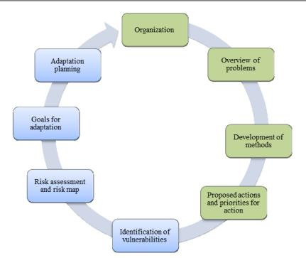
Fig. 7. Eight steps in developing an adaptation plan for the adaptation of road drainage structures to climate change. (Green boxes: steps elaborated upon in the text).
