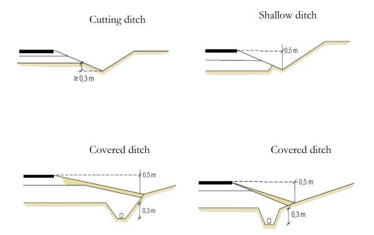
Fig. 2. The most common types of dewatering ditches in Sweden (redrawn from Lind et al., 2003, with permission from STA).
