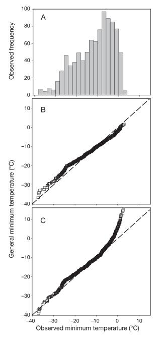
Fig. 1. Comparison between generated and observed minimum temperatures for the LARS-WG stochastic weather generator versions 5.0 and 4.0 for January at Kuopio, Finland. (A) Frequency distribution for observed daily minimum temperature, (B) Q-Q plot of generated vs. observed minimum daily temperature for LARS-WG 5.0 and (C) Q-Q plot for LARS-WG 4.0
