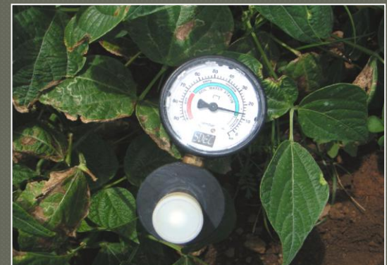
Use of Tensiometers, to monitor soil moisture for irrigation scheduling
