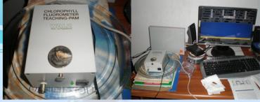
Figure 2.0: Pulse-Amplitude-Modulated (PAM) fluorometer
