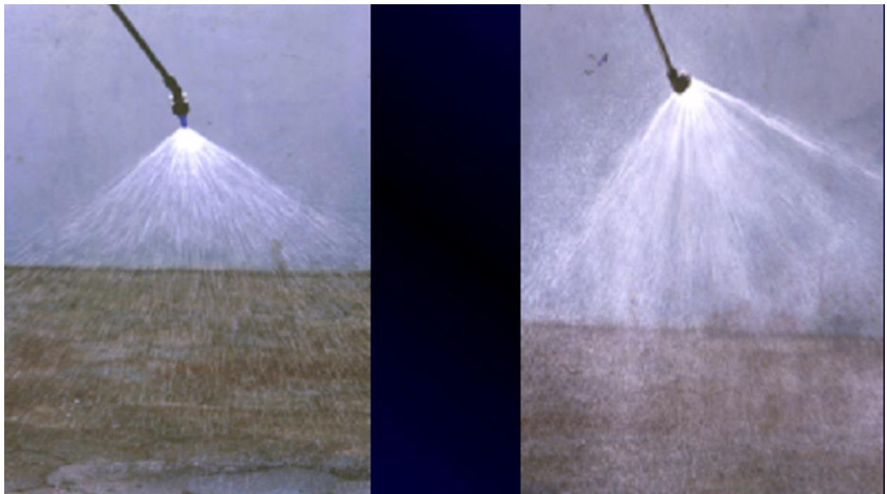
Figure 4. Very few small droplets with air-inclusion nozzle (left) than with conventional flat-fan nozzle (right), greatly reducing drift (Source; MSIRI).
