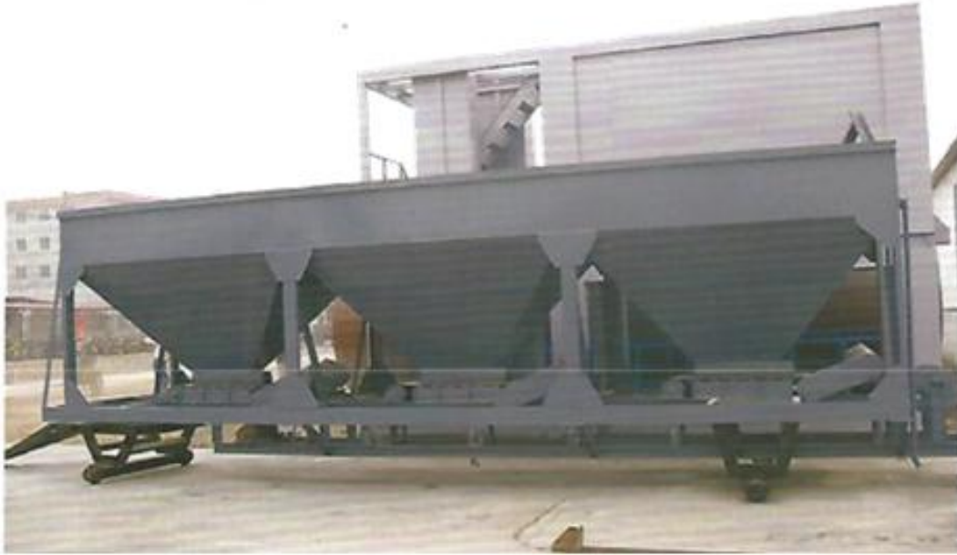
Figure 4: The cold feeder system
