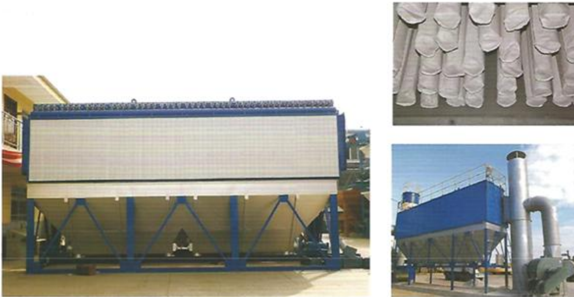
Figure 7: The drying system – Baghouse dust collector
