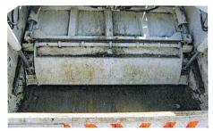
A hydraulic compacting device
