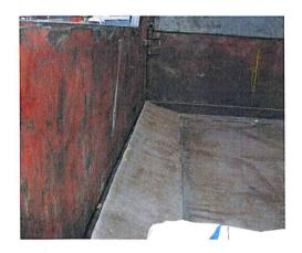
Proper leachate retaining device to be fixed at the bottom of the basket.Dimension of leachate retaining device- (3 inches x 6 inches) at the rear of lorry basket and (3 inches x 3 inches) on the right / left side of the lorry basket.
