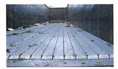
Moving floor made up of metal blades with sliding movements. Rubber seal provided between blades.
