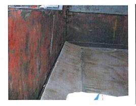
Proper leachate retaining device to be fixed at the bottom of the basket. Dimension of leachate retaining device- (3 inches x 6 inches) at the rear of lorry basket.
