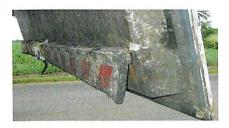
A rubber seal available at bottom and sides edges of rear door.
