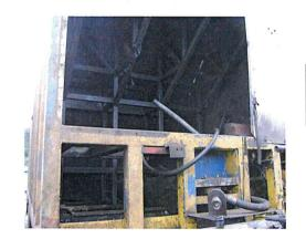
A hydraulic ejecting device for the unloading of wastes.
