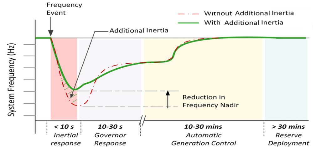
**NEED TO COMPENSATE FOR REDUCTION IN INERTIA**
