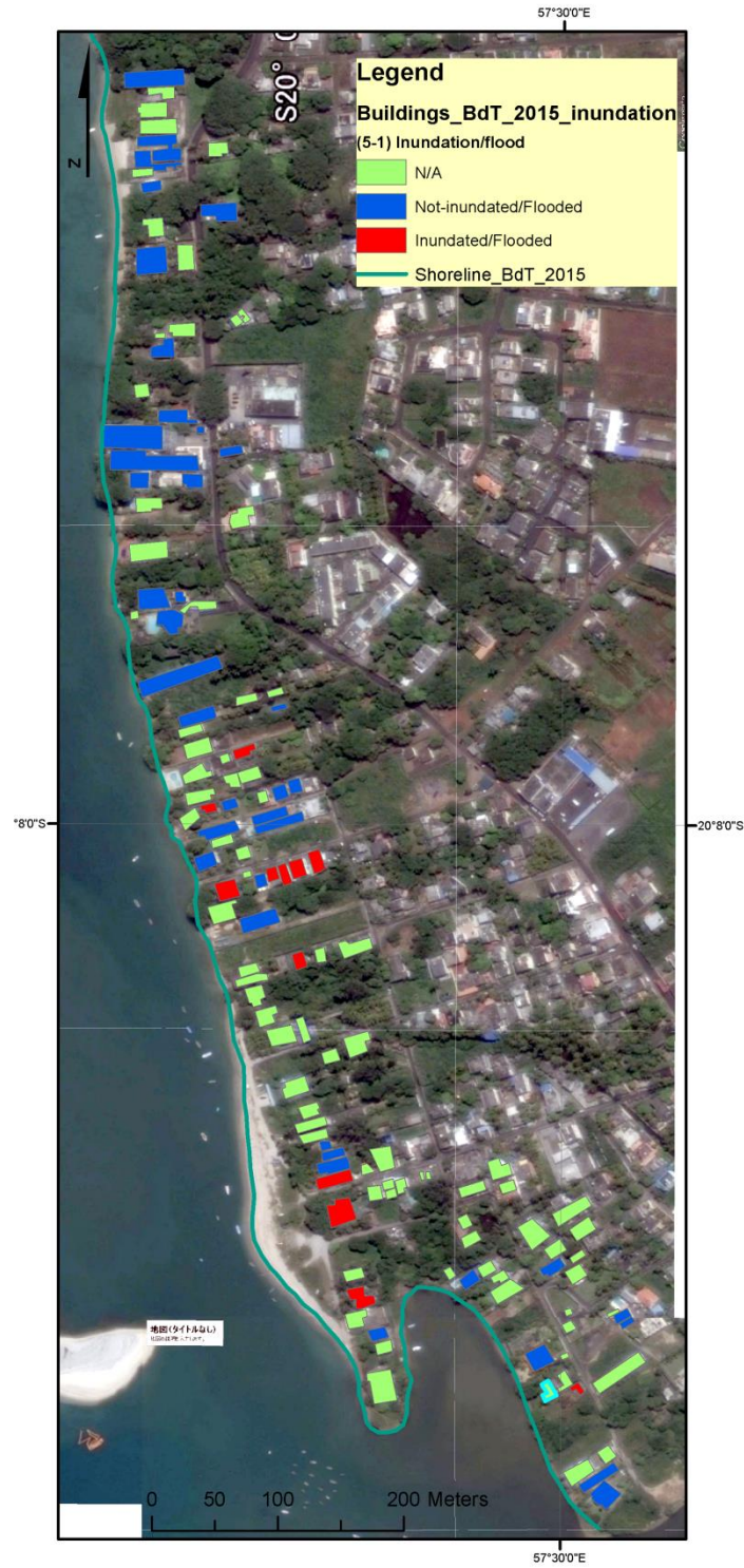
Figure : Buildings situated within 100m from shoreline and being affected or not by inundation
