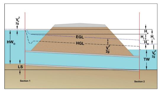
Figure 3.8. Full flow energy and hydraulic grade lines.
