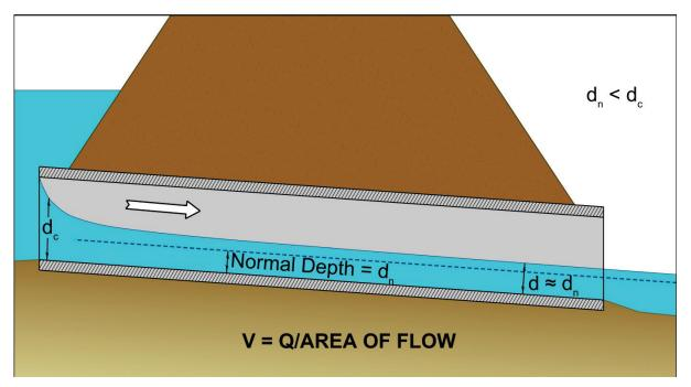
Figure 3.13. Outlet velocity - inlet control.
