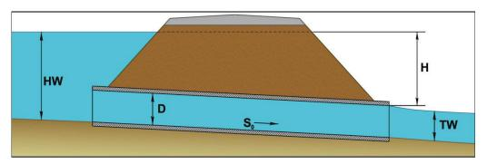
Figure 3.29. USGS flow type 4 and 6.
