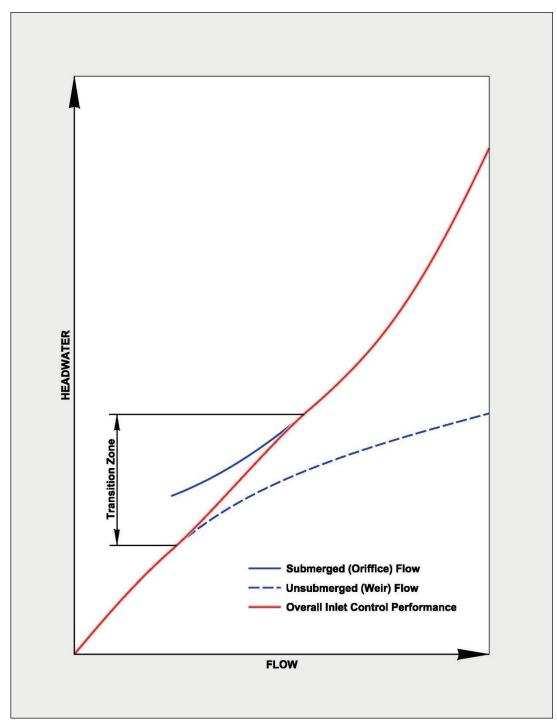
Figure 3.4. Inlet control curves.
