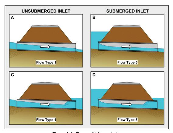
Figure 3.1. Types of inlet control.
