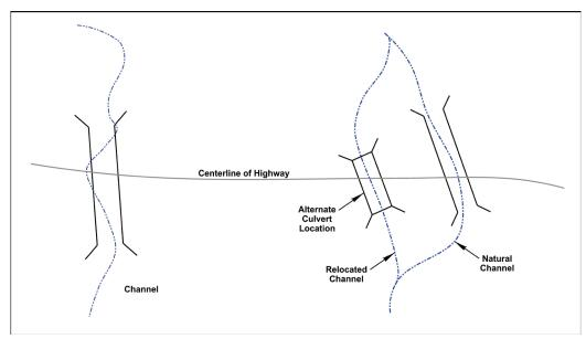
Figure 2.3. Culvert location methods.
