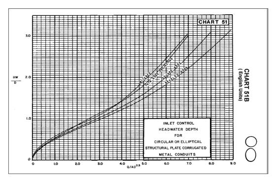
Figure 3.31. Inlet control curves - circular or elliptical structural plate corrugated metal conduits (Chart 51B).
