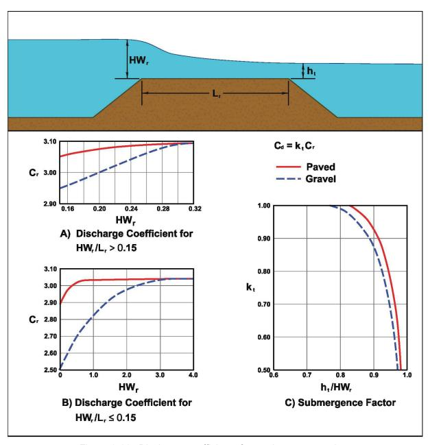
Figure 3.11. Discharge coefficients for roadway overtopping.
