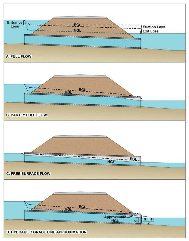
Figure 3.9. Outlet control energy and hydraulic grade lines.
