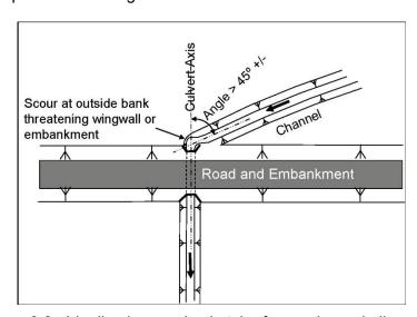
Figure 6.6. Idealized example sketch of poor channel alignment.
