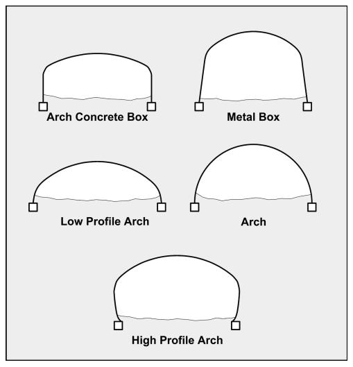
Figure 1.5b. Commonly used open-bottom culvert shapes.
