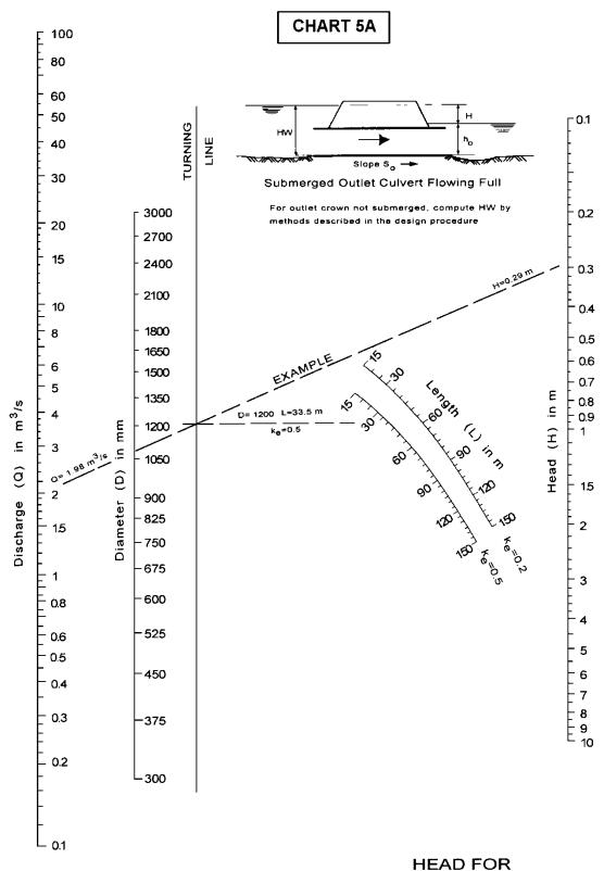
CONCRETE PIPE CULVERTS FLOWING FULL n=0.012
