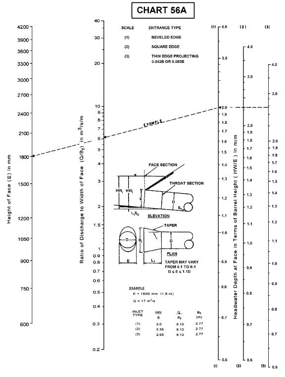
FACE CONTROL FOR SIDE-TAPERED INLETS TO PIPE CULVERTS (NON-RECTANGULAR SECTIONS ONLY)
