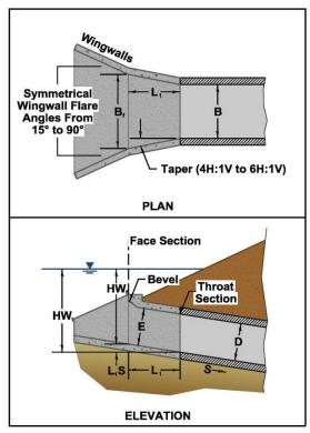
Figure 3.19. Side-tapered inlet.
