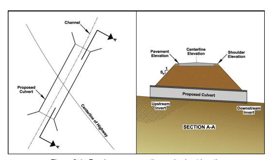
Figure 2.4. Roadway cross section and culvert length.
