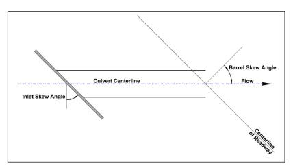
Figure 5.14. Inlet skew angle.
