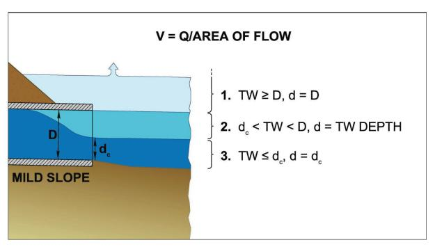
Figure 3.14. Outlet velocity - outlet control.
