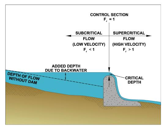
Figure 1.16. Flow conditions over a small dam.
