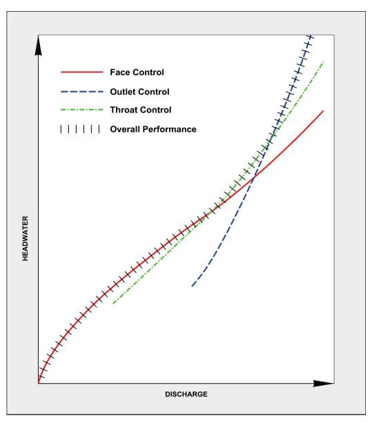
Figure 3.23. Culvert performance curve.
