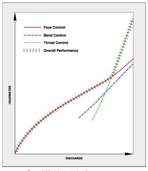
Figure 3.22. Inlet control performance curves.
