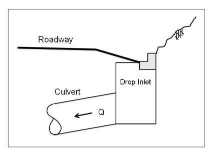
Figure 5.8. Drop inlet to straight culvert.
