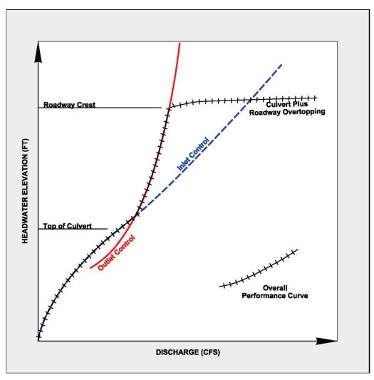
Figure 3.16. Culvert performance curve with roadway overtopping.
