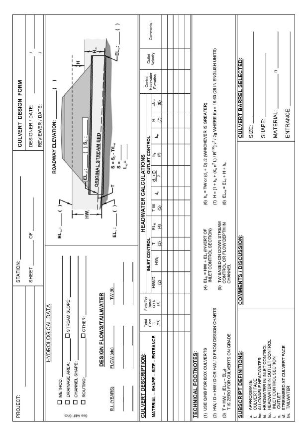
Figure 3.17. Culvert design form.
