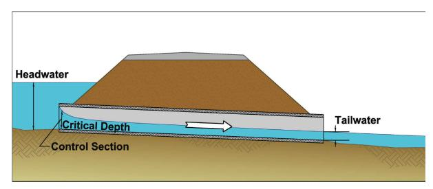
Figure 1.17. Typical inlet control flow section.
