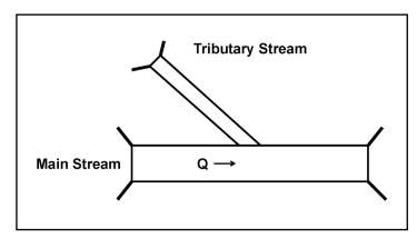
Figure 5.4. Culvert junction.
