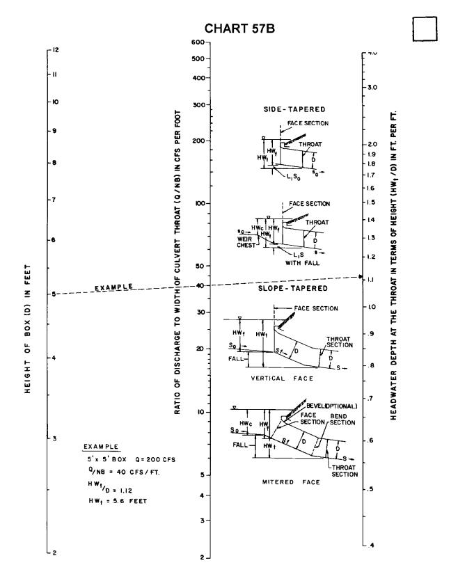
THROAT CONTROL FOR BOX CULVERTS WITH TAPERED INLETS
