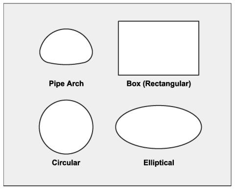
Figure 1.5a. Commonly used culvert shapes.
