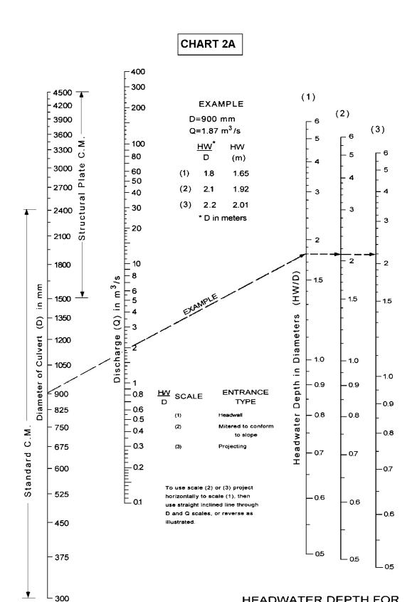
Adapted from Bureau of Public Roads Jan. 1963 HEADWATER DEPTH FOR C.M. PIPE CULVERTS WITH INLET CONTROL
