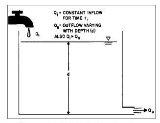
Figure 5.24. Hole in the barrel analogy.
