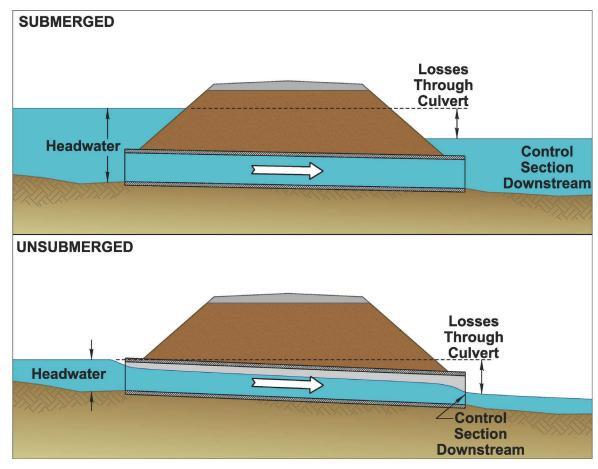
Figure 1.18. Typical outlet control flow conditions.
