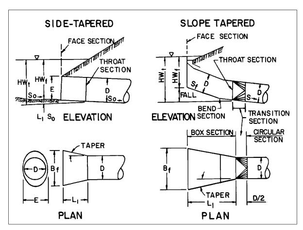
Figure DG 3.2. Tapered inlets for pipe culverts.
