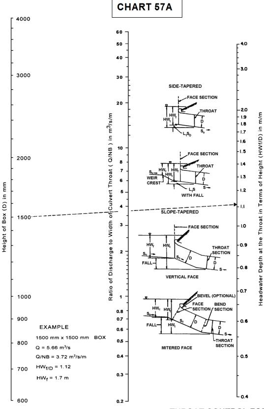
THROAT CONTROL FOR BOX CULVERTS WITH TAPERED INLETS
