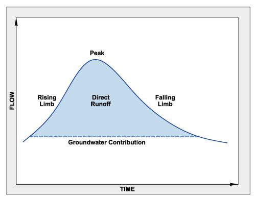
Figure 2.1. Flood hydrograph.
