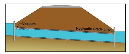
Figure 5.5. Subatmospheric pressure in culverts.
