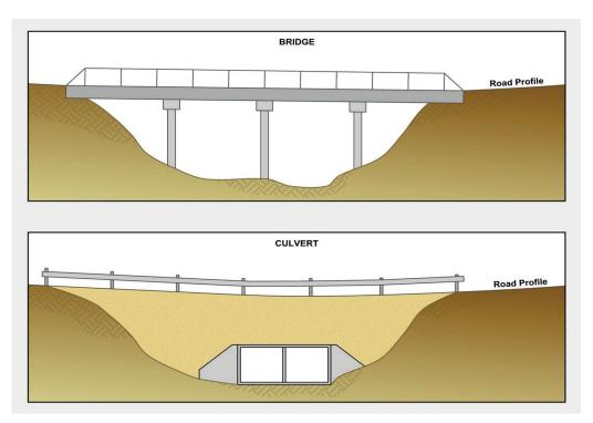
Figure 1.4. Bridge versus culvert at same location.
