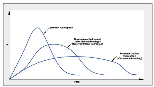
Figure 2.2. Flood hydrograph shape modification.
