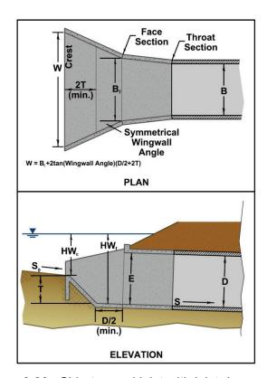
Figure 3.20. Side-tapered inlet with inlet depression.
