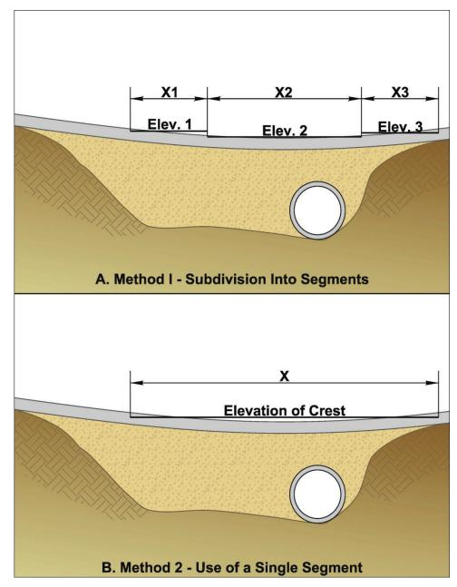
Figure 3.12. Weir crest length determinations for roadway overtopping.
