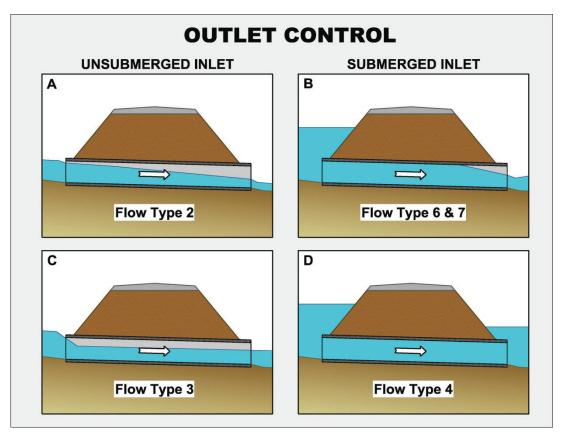
Figure 3.7. Types of outlet control.
