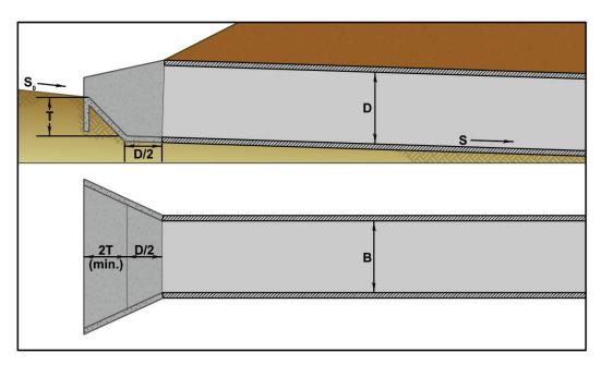
Figure 3.5. Culvert with inlet depression and with apron and wingwalls.
