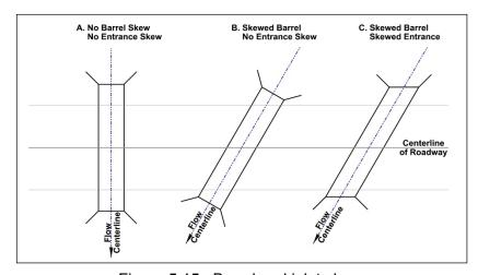
Figure 5.15. Barrel and inlet skew.
