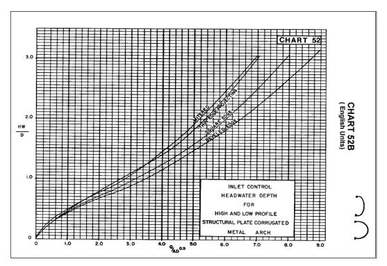
Figure 3.32. Inlet control curves - high and low profile structural plate arches (Chart 52B).
