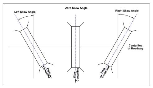
Figure 5.13. Barrel skew angle.
