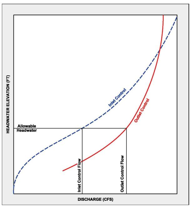
Figure 1.19. Culvert performance curve.
