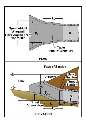
Figure 3.21. Slope-tapered inlet with vertical face.
