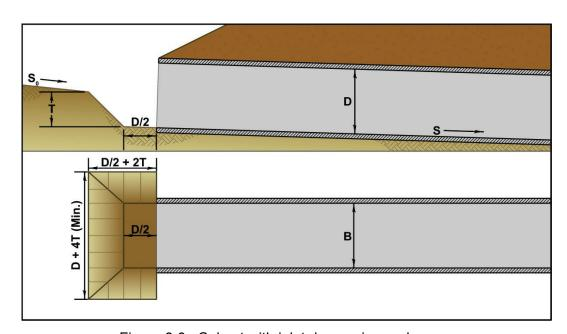
Figure 3.6. Culvert with inlet depression and sump.
