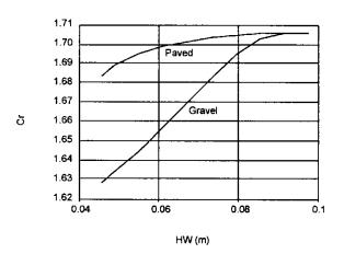
A) Discharge Coefficient for HWr/Lr > 0.15
