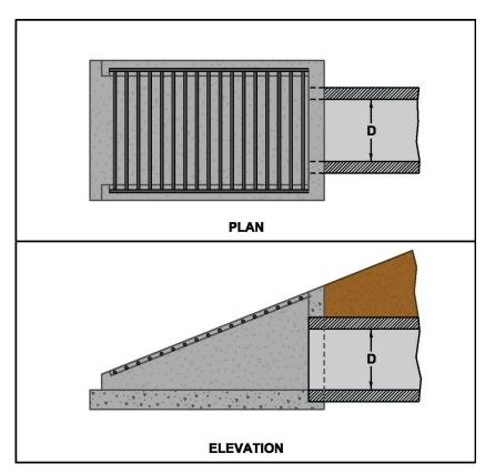
Figure 2.10. Endwall for safety grate.
