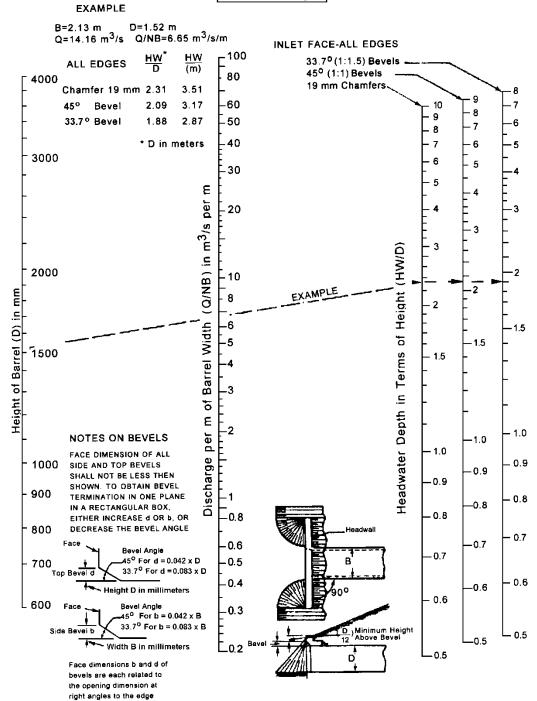
Adapted from Federal Highway Administration May 1973 HEADWATER DEPTH FOR INLET CONTROL RECTANGULAR BOX CULVERTS 90° HEADWALL CHAMFERED OR BEVELED INLET EDGES
