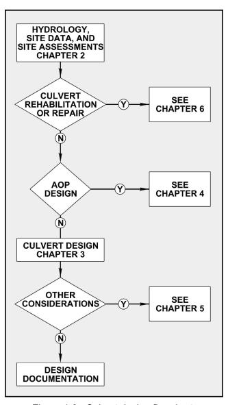
Figure 1.3. Culvert design flowchart.
