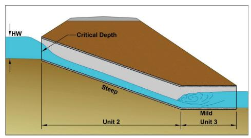
Figure 5.23. Two-unit broken-back culvert.
