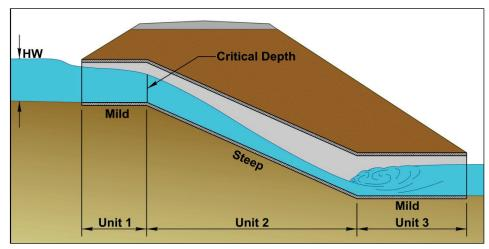
Figure 5.22. Three-unit broken-back culvert.
