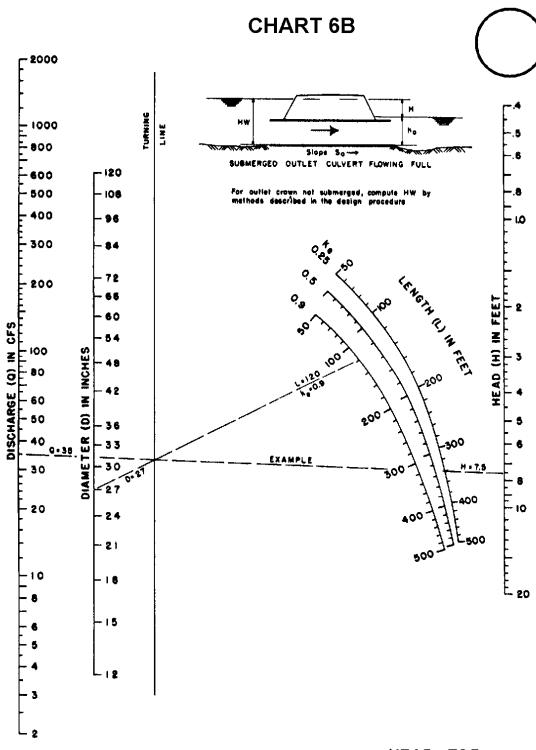
HEAD FOR STANDARD C. M. PIPE CULVERTS FLOWING FULL n = 0.024
