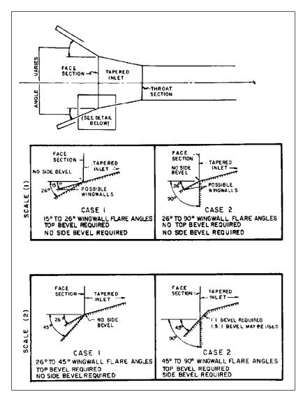
Figure DG 3.1. Inlet edge conditions, face section, rectangular tapered Inlets.
