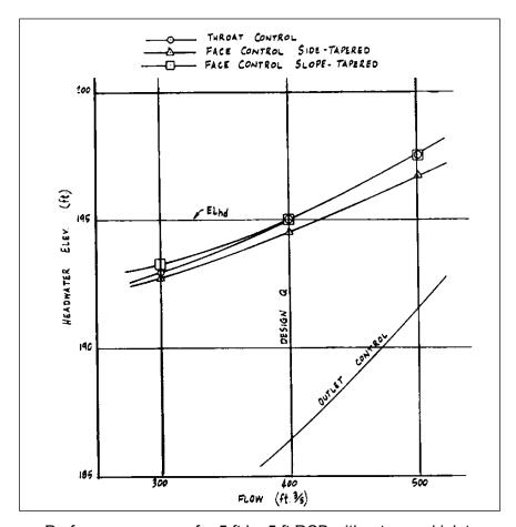
Performance curves for 5 ft by 5 ft RCB with a tapered inlet.
