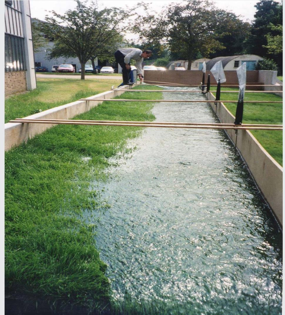
Testing in PRG channel;  $Q = 50.8$  l/s; grass height = 100mm
