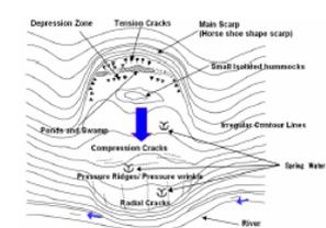
Schematic diagram of landslide landforms
