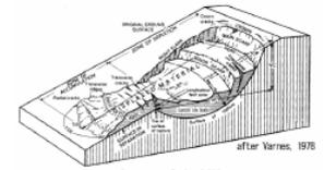
Structure of a landslide
