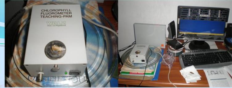
Figure 2.0: Pulse-Amplitude-Modulated (PAM) fluorometer
