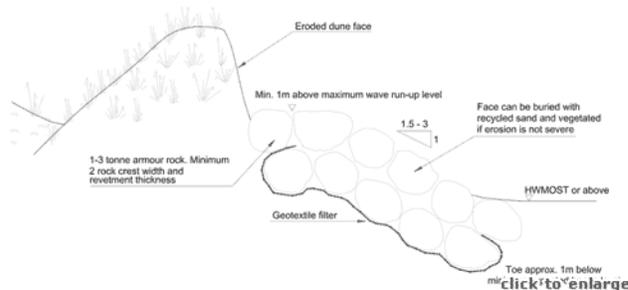
Cross-sectional view of revetment.
