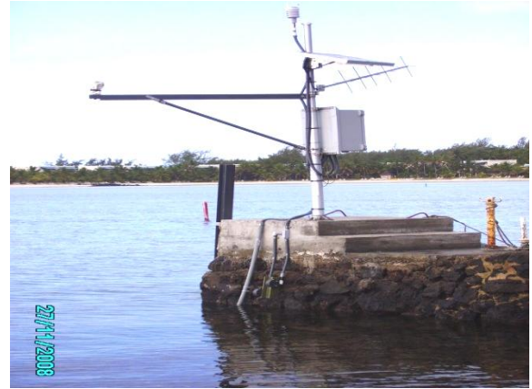
Figure 6.4 - An automatic weather station and, a tide gauge (right). (Courtesy : MMS)
