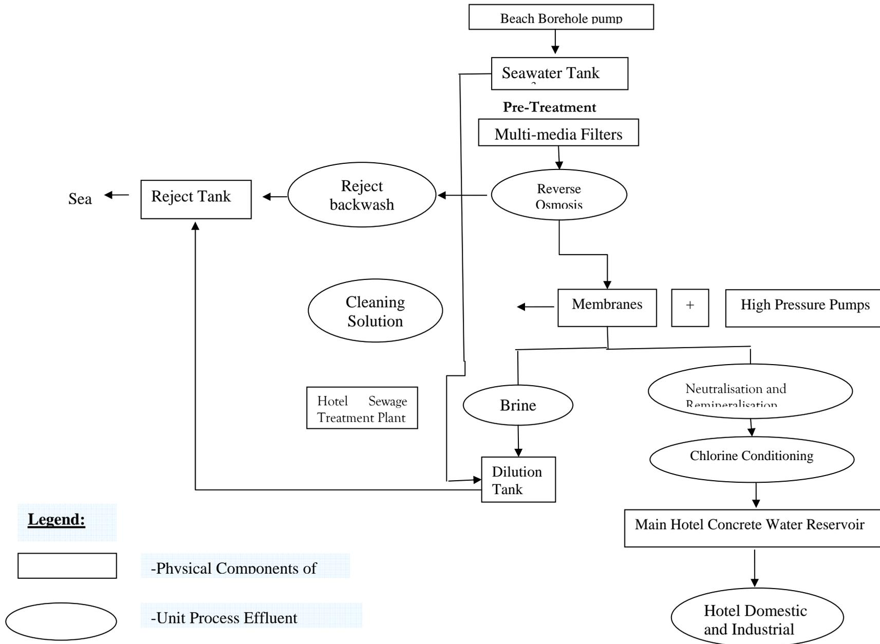
**Figure 7-5: Detailed Flowchart of Proposed Seawater Desalination Facility**
