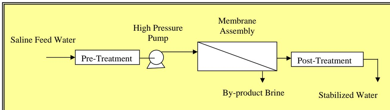
**Figure 7-1: Basic Process Flow Diagram**
