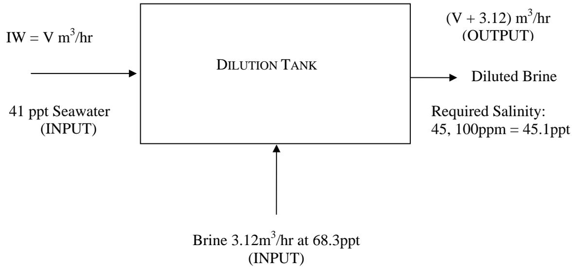
**Figure 7-4: Computation of Required Flowrate from Beach Intake Borehole for Brine Dilution**
