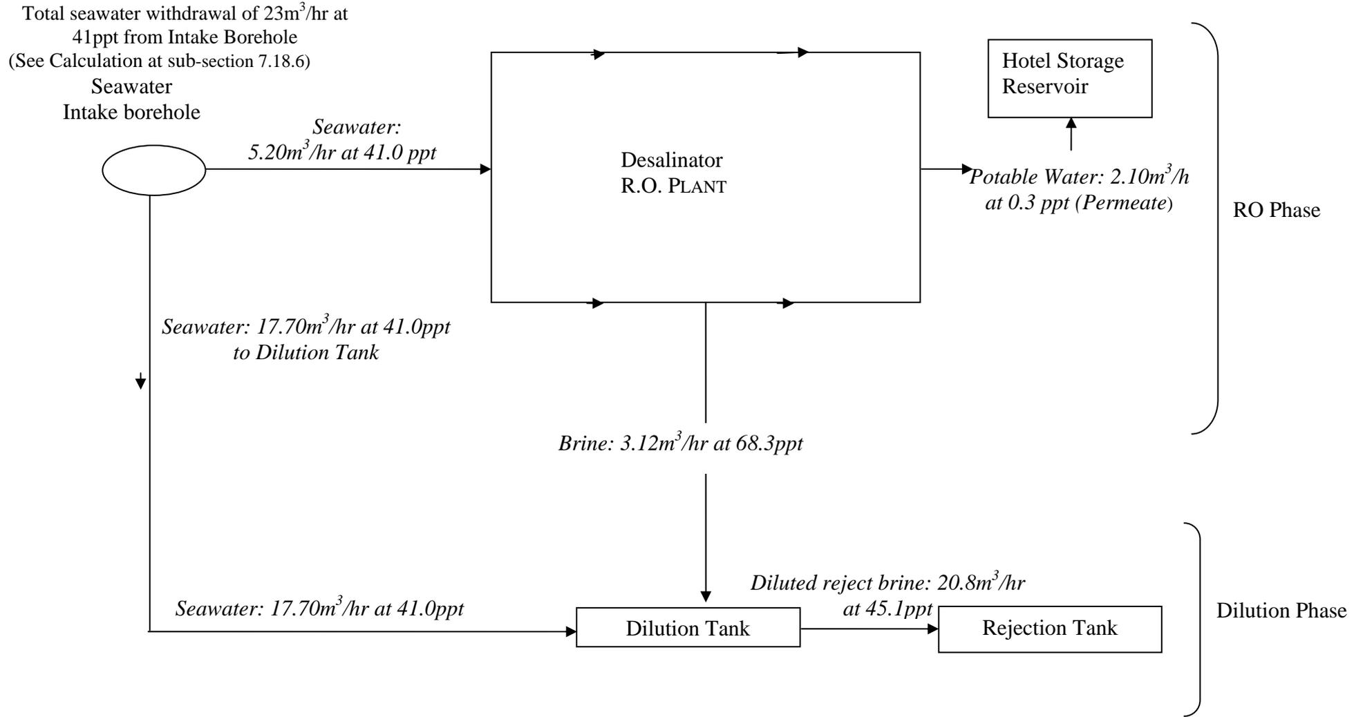
Figure 7-3: Entire Desalination Process Mass Balance Diagram
